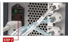
\*Flip the switch **off** at the back of the machine.
