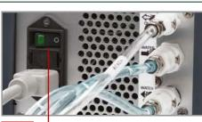
STEP 2 \*Flip the switch off at the back of the machine. \*Important: Do not switch off in the back before turning off the front of the unit
